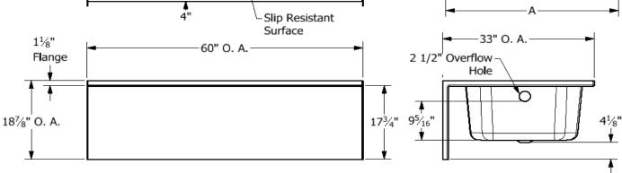
Certified to conform to HUD/UM73b,ANSI Z124.1, and ASTM E- 162 Flame Spread Rating 200 or less and is under a program of factory inspection.
